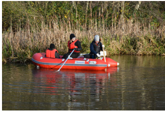
Figure 2.2: Fixing position with wooden pole, recording GPS-coordinates and water depth.
