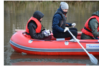
Figure 2.4: Recording GPS-coordinates (Latitude and Longitude) and water depth in field book.
