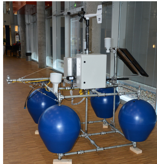
Figure 5.2: Assembled automatic climate and water monitoring station ready for application in Kvaglund lake - different angle.
