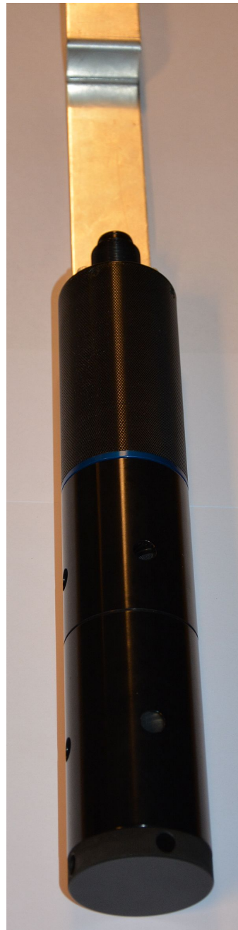
Figure 3.26: Aquaread probe AP-5000 with protective cover to protect the sensors and electrodes.
