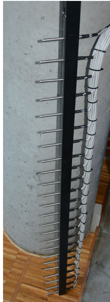
Figure 3.22: Temperature array measurement using 24 PT-100 sensors with an equidistant 5 cm spacing to measure the vertical temperature profile in each lake.
