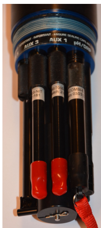
Figure 3.24: Individual optical sensors and electrodes mounted to the Aquaread AP-7000 probe.
