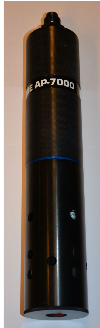
Figure 3.23: Aquaread probe AP-7000 with protective cover to protect the sensors and electrodes.
