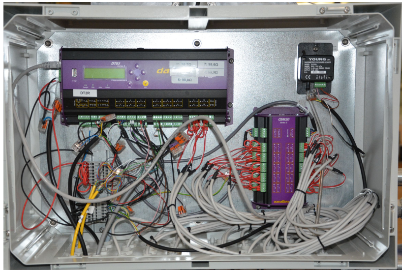
Figure 3.13: Data logger DT85 and channel extension module CEM20 installation in data logger box. All cables connected to the data logger and CEM20 module passing through water tight fittings in the bottom of the data logger box to the individual sensor.
