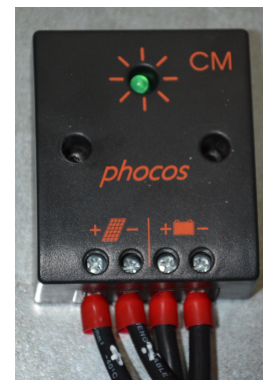
Figure 3.10: Charge regulator ensuring that the battery is recharged when ever sufficient sunlight is available and preventing the battery from overcharging.
