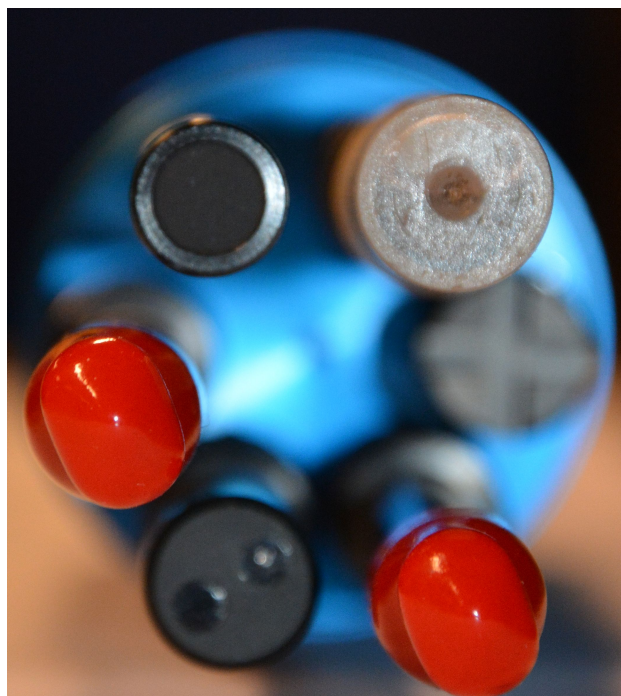
Figure 3.28: Bottom view on mounted optical sensors and electrodes.
