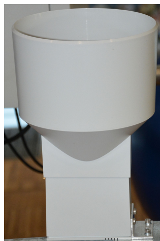
Figure 3.20: Rain gauge sensor to measure precipitation.
