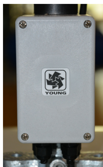
Figure 3.16: Young compass (model 32500) to determine reference north for calculating correct wind direction.
