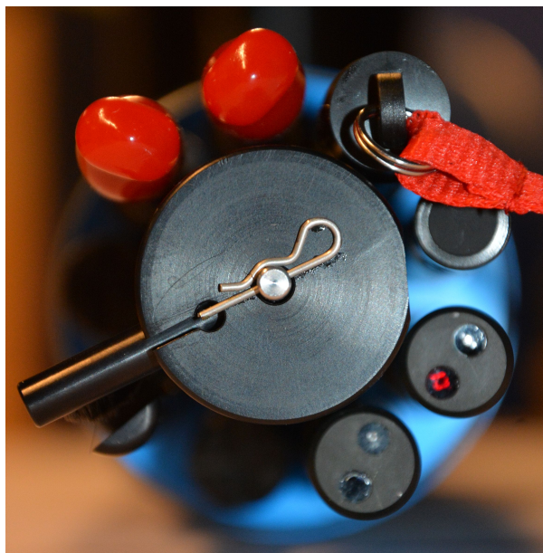
Figure 3.25: Bottom view on mounted optical sensors and electrodes as well as cleaning brush.
