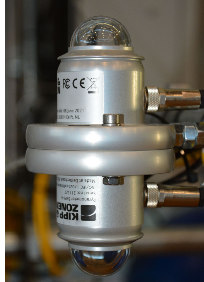
Figure 3.21: Albedometer measuring incoming and reflected solar radiation.
