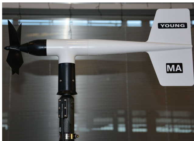
Figure 3.15: Wind speed and wind direction measurement sensor Young Wind Monitor - MA (model 05106).
