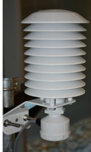
Figure 3.17: Air temperature and humidity measurement sensor.
