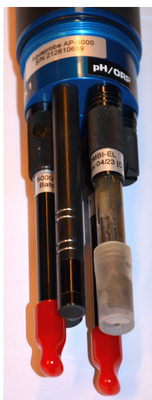
Figure 3.27: Individual optical sensors and electrodes mounted to the Aquaread AP-5000 probe.
